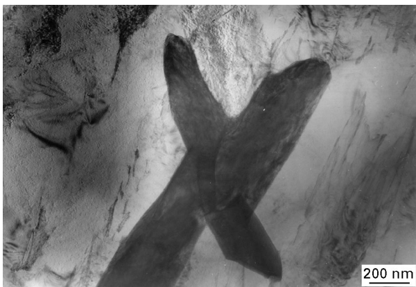
Figure 2 Bright-field transmission electron micrograph of two or three needles being almost in the same diffraction condition.
